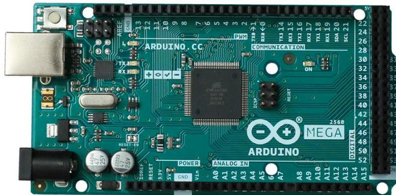
*Fig 3.1 Arduino Mega 2560 rev3*
