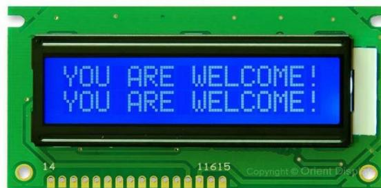
*Fig 3.5 LCD Display*
